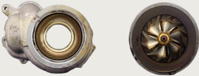
Images show BMW turbo-charger unit from N20 engine
